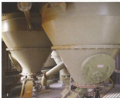
Two of the four fluidized blending tanks which make up the dual in-line blending system
